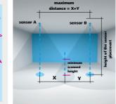
Suitable placement of presence detectors with partial overlap of scanned areas
