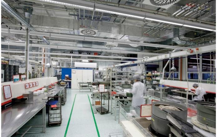
demanding visual tasks require In the premises typical for increasing the level of the mini- high dustiness, it is necessary mal illuminance to 1.500 lux. It can be achieved by installing an additional luminaire directly towards the task area. The higher level of illuminance will enable the employee to perceive the contrast better and will improve corrosion. When solving the his/her 3D perception.
