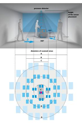
Direct walking Perpendicular walkina Working position Presence detector
