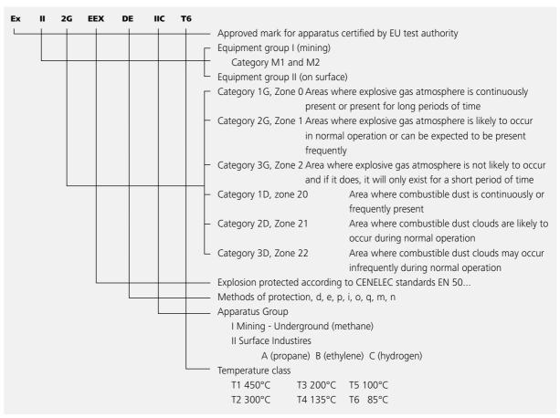
Methods of protection: Flameproof Type of Protection "d"- or Explosionproof Equipment
