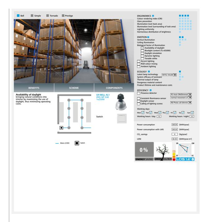
The space is illuminated by luminaires The area of ecology represents a equipped with high-pressure metal--halide lamps 250 W. It is a suspended rotationally symmetric lighting fixture. This type of luminaire achieves lifespan and also high maintenance as the lighting uniformity which helps us achieve good results of the ergonomic parameters.
