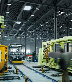
In the production halls of the automotive industry the Paintshop is a space which places specific demands on the lighting solution. The standard EN 12464-1 states the Some operations in the paintminimal illuminance level 750 lux for the paintshops (1,000 lux for the touch-up the direct distribution of the luminous flux and additional luminaires with a distinctively asymmetric luminous intensity curve by which we can achieve
