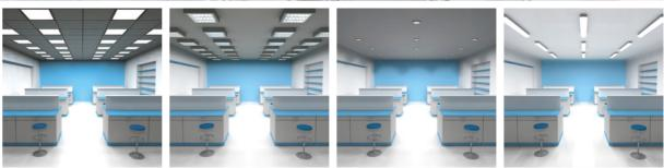
The harmonious distribution of brightness in a space can be influenced by a selection of luminaires. By using luminaires with direct distribution of the luminous flux (Figure 1-3) we don't achieve sufficient illuminance of vertical surfaces, which causes a cave effect. It can be avoided by using luminaires with a very wide luminosity curve. (Fig. 4).
