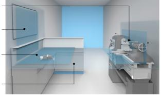
Various industrial workplaces require different lighting solutions for individual visual tasks. These must be defined individually in terms of location and intensity of illumination. The individual tasks may be combined and performed in the same working area.
