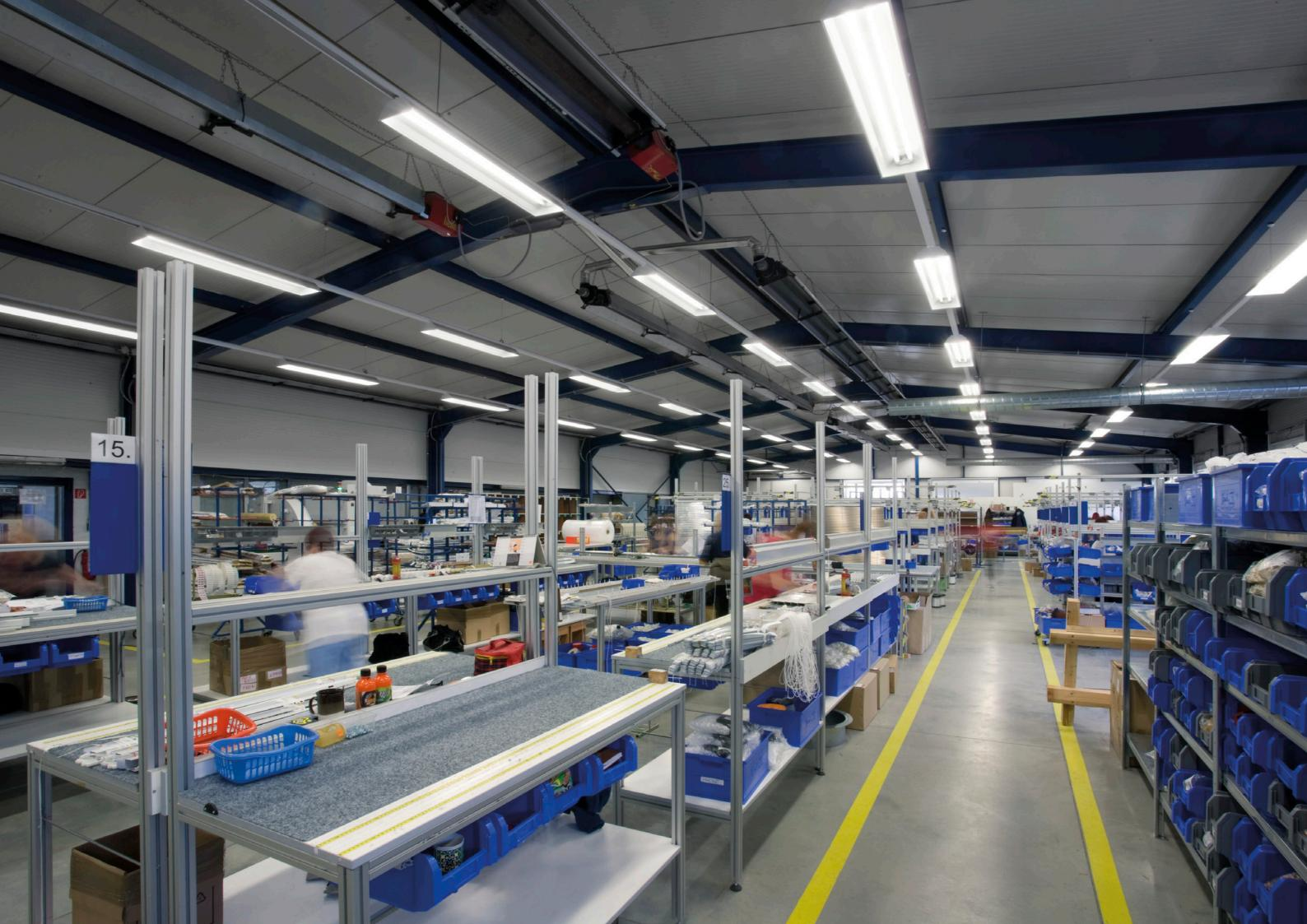
If an excessive amount of dust develops during this type of production, it is recommended to use the luminaires with the higher-degree protection.
