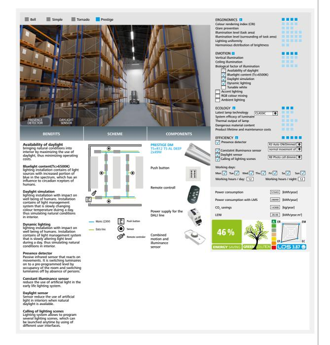
We achieved the required space illuminance by using the suspended luminaires with the direct characteristic of the luminous flux distribution with FHD (T5) light sources 2x49 W. The light curve is shaped in such a way that we will achieve the necessary vertical illuminance of the racks in the warehouses and at the same time also sufficient horizontal illuminance of the task area.
