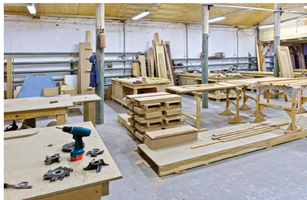
When solving the lighting system in the woodworking and processing industry it is necessary to avoid the stroboscopic effect when the artificial lighting is on. The stroboscopic effect represents a serious danger especially when the employee works with rotational tools.
