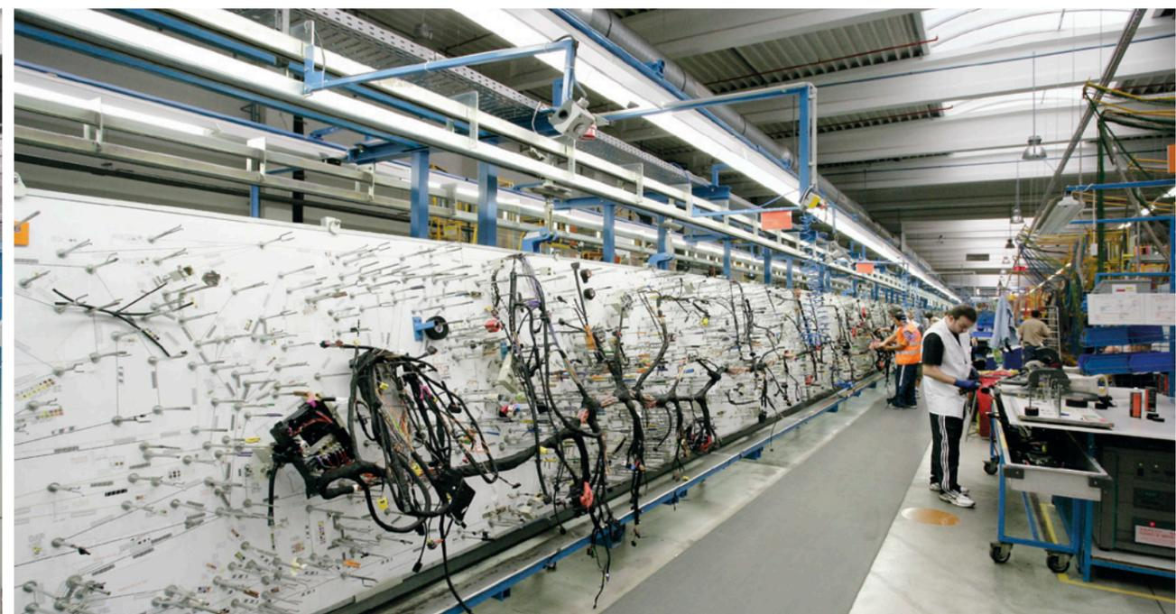
demanding visual tasks require increasing the level of the minimal illuminance to 1,500 lux. It can be achieved by installing an additional luminaire directly towards the task area. The higher level of illuminance will enable the employee to perceive the contrast better and will improve his/her 3D perception.
