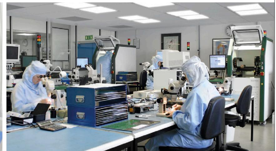
Luminaires for the cleanroom should be produced from a material with low porosity which even after contacts with chemicals does not change its properties.
