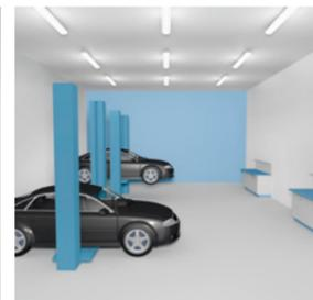
*In production halls with standard height of the walls it is suitable to use linear luminaires with the direct characteristic of the luminous flux. To obtain the standard stated levels of the maintained illuminance it production halls with non standard height of the walls (6 m and more) it is important to choose luminaires that can be used in different mounting height*
