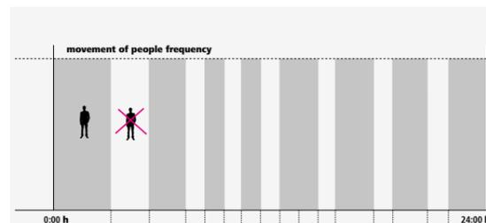
**Regulation in leaps:** When presence is detected, the luminaires turn on in leap only when illumination level is lower than the preset value. If the illuminance is higher, luminaires in the room remain off even if movement continues. For this type of combined lighting management system luminaires do not need to be equipped with dimmable control gear power components.
