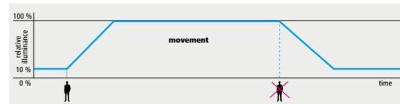
Time procedure of presence detector - without delay
