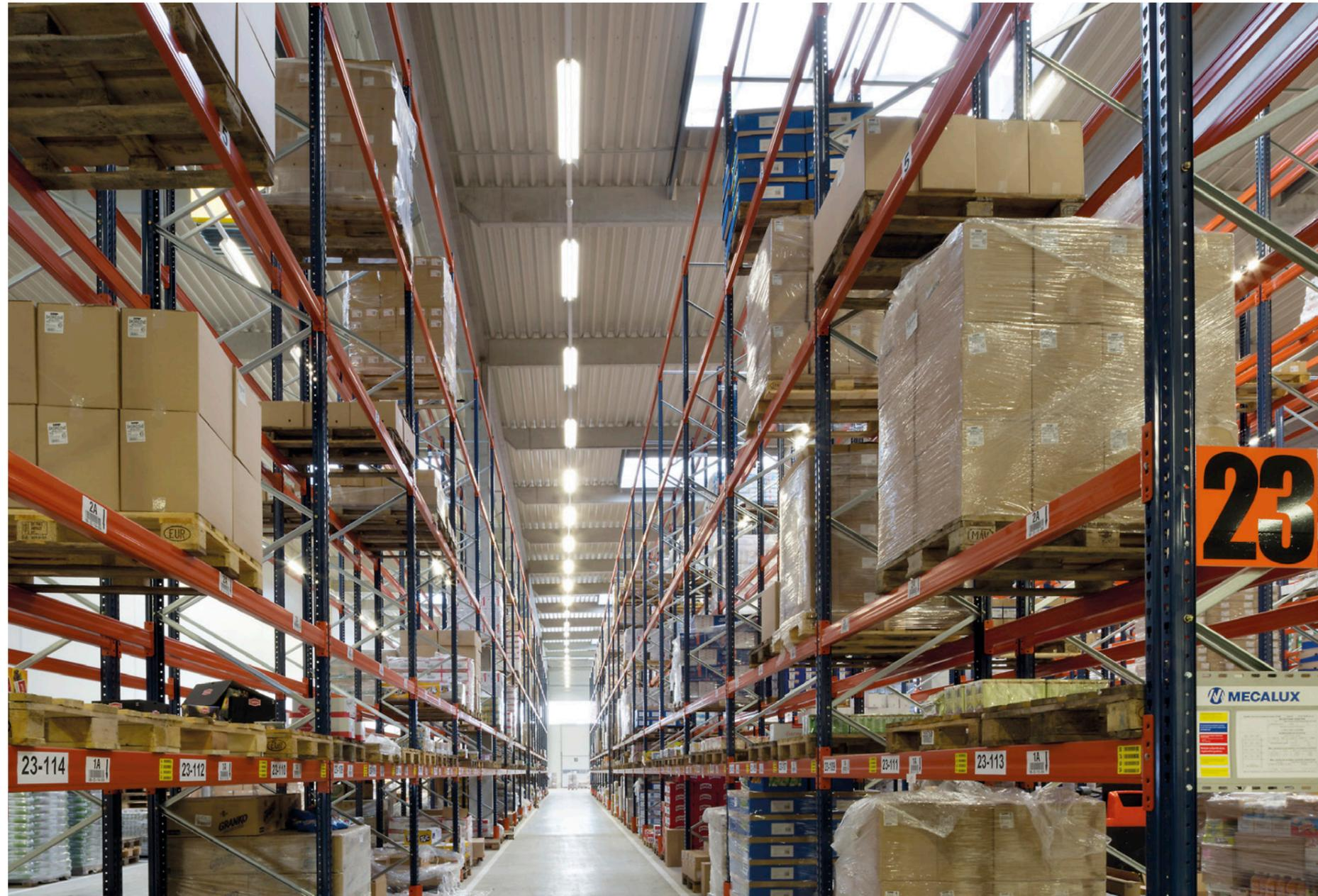
high-positioned racks in the halls with the wall height 6 metres and more, it is suitable to use the high-bay reflector luminaires with asymmetrical reflectors fitted with housing which will prevent direct glare of the employees when they look directly upwards. Besides the required level of the maintained illuminance it is simultaneously possible to achieve the uniform distribution of the luminance in the warehouse premises with both lighting solutions.
