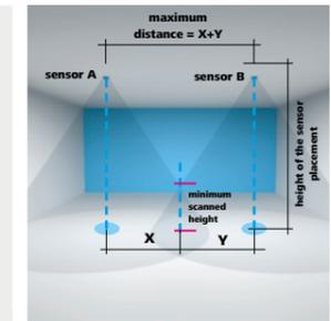
Suitable placement of presence detectors with partial overlap of scanned areas
