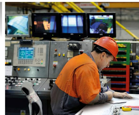
The optimal solution is considered when the luminaire is placed towards the working surface slightly from the left of the employee's view. When the situation is solved like this the employees do not cast a shadow upon the desk when they are working and also good visibility of the working tool's spike or pen's nib is ensured.
