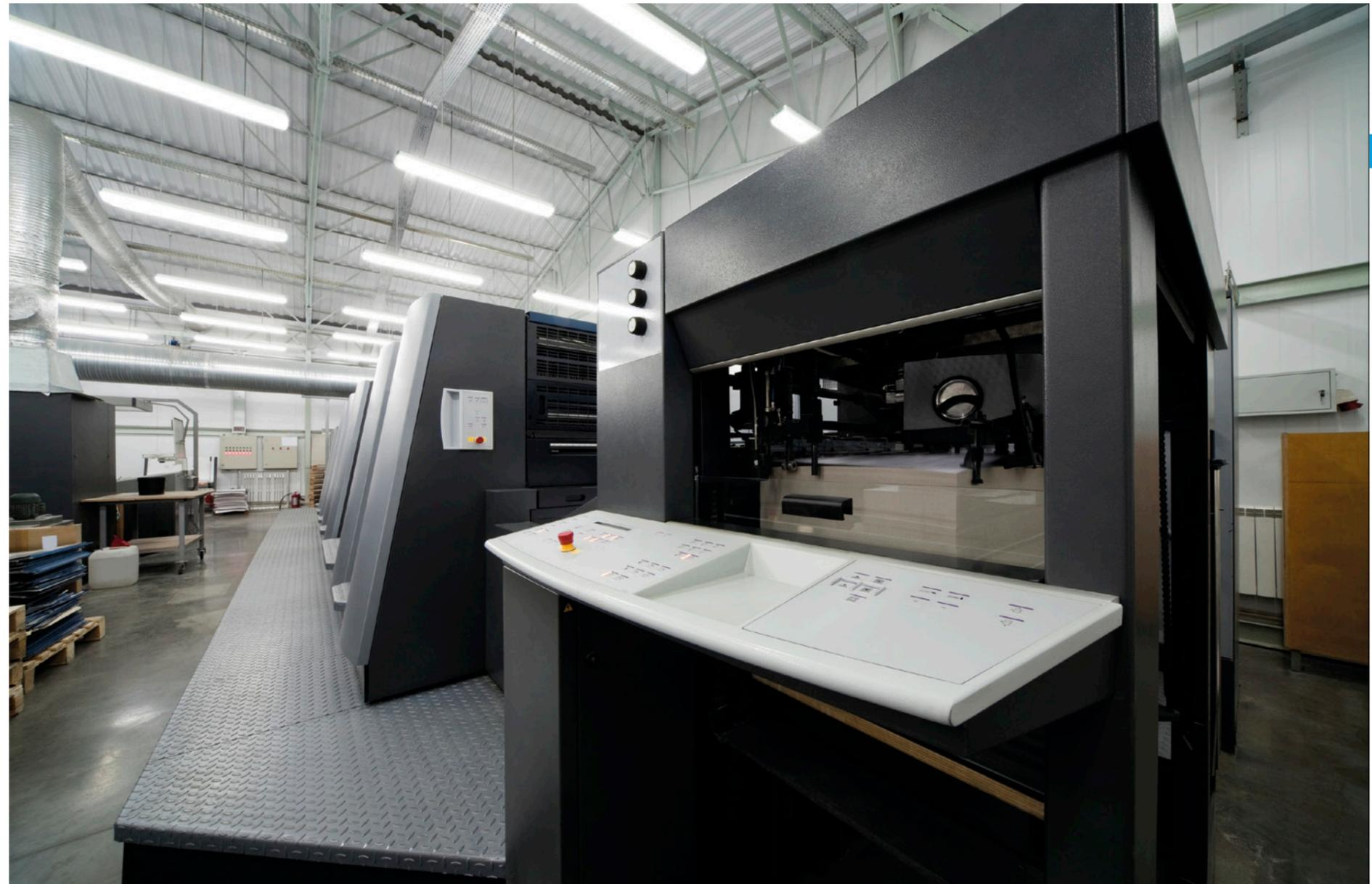
For the multicolour printing process and the inspection operations it is necessary to use the light sources with the colour rendering index  $CRI \geq 90$  for correct distinguishing of colours.
