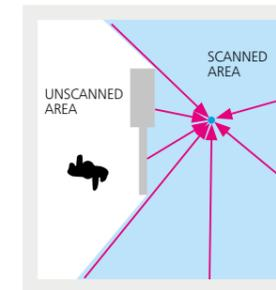
Scanned area of passive infrared sensor (PIR)
