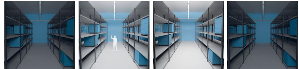
If in the scanned area no movement of an employee has been detected, the luminaires remains on low illumination level (safety reasons).
