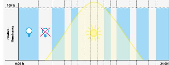
**Continuous regulation:** When presence is detected, the luminaires turn on, followed by a continuous adjustment of desired level based on scanning of illuminance in area. If the movement persists, the luminaires are dimmed up and down according to requirements on illuminance level. For this type of combined lighting management system must be luminaires equipped with dimmable control gear power components.
