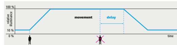
Time procedure of presence detector - with delay
